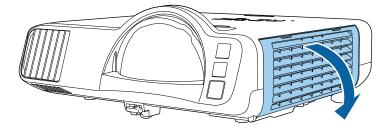
**3** Pull the air filter out of the projector.
