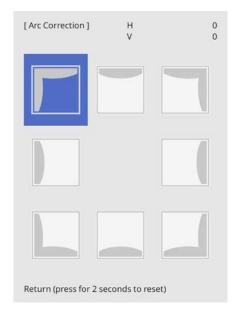
**8** Press the arrow buttons to adjust the image shape of the selected area as necessary.
